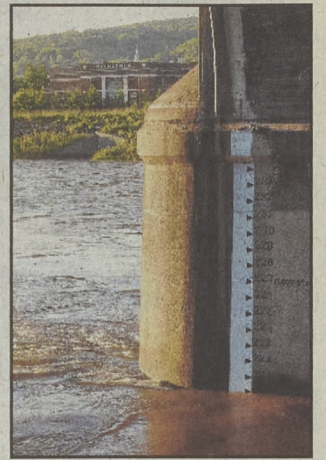
The Hill-to-Hill bridge Lehigh River depth measurement recorded 20 feet at 7 p.m. Monday morning, which put the river at seven feet below the 28-foot flood mark.
