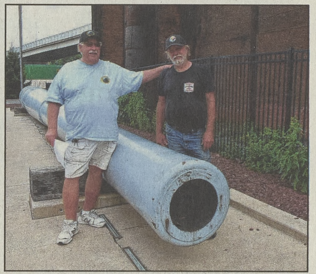
Bethlehem Steel tour guides from left, John Weiss and Joe Mayer, both former steelworkers, provide insight into the "Steel" portion of the morning's journey. Here they tell the story of a 60-foot, 188,000-pound gun manufactured at the high house behind them for the battleship USS Mississippi in 1919. The gun could fire a 14-inch diameter shell that weighed 1,800 pounds. The projectile could travel for up to 20 miles.
