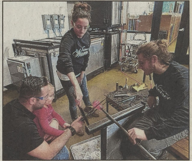
As Warner volunteer Dan Polk turns the pipe, Mackenzie and her dad use jacks to create a paperweight from the molten glass with steady assistance from Melinda Wolterman and her paddle. The groove will be where the piece breaks off from the pipe.
