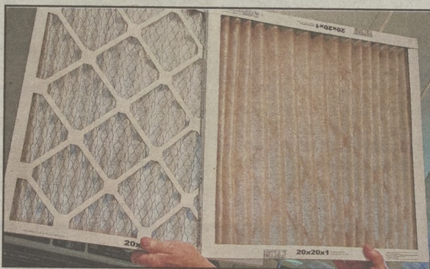
Installing a fresh furnace filter is one way to ensure the furnace runs smoothly through the winter.
