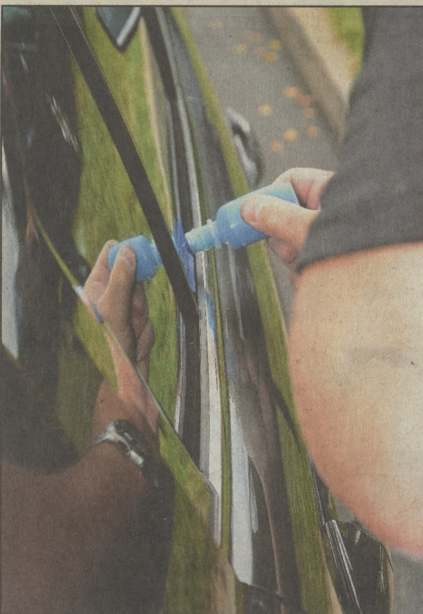
A detective applies acid over the stencil to etch the VIN number on the window.
