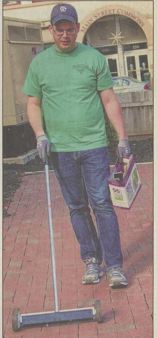
Todd Dietrich pushes a magnetic roller device to pick up screws, nails and other metallic junk in the Sun Inn brick courtyard along Main Street in downtown Bethlehem.
