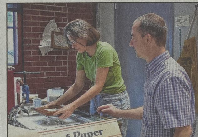
Amy Capwell creates a liquid sheet of paper as she pulls a deckle up out of a sink full of paper pulp while being coached by papermaking expert Tom Necker.
