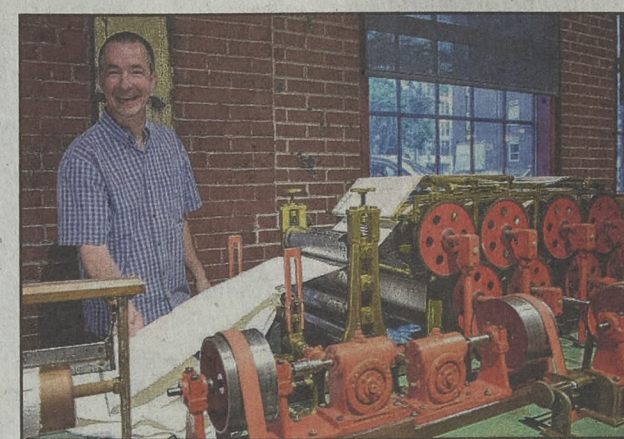
Papermaking expert Tom Necker is pleased with the continuous roll of paper piling off the scale model of a Rice, Barton, and Fales Fourdrinier Paper Making Machine.
