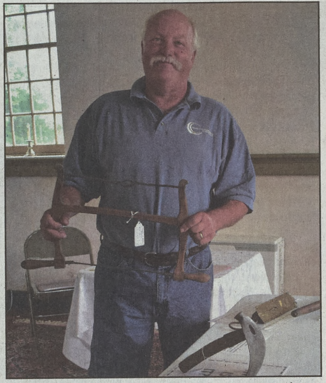
Society member Bob Swan picks up an antique hand saw from a collection of vintage tools on display. Swan explains that the tool is also known as a buck saw or bow saw.
