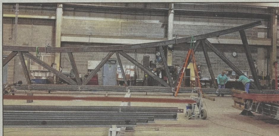
COURTESY OF LEVAN ASSOCIATES INC. STEEL FABRICATOR AND ERECTOR A gym truss being welded in the Levan shop
