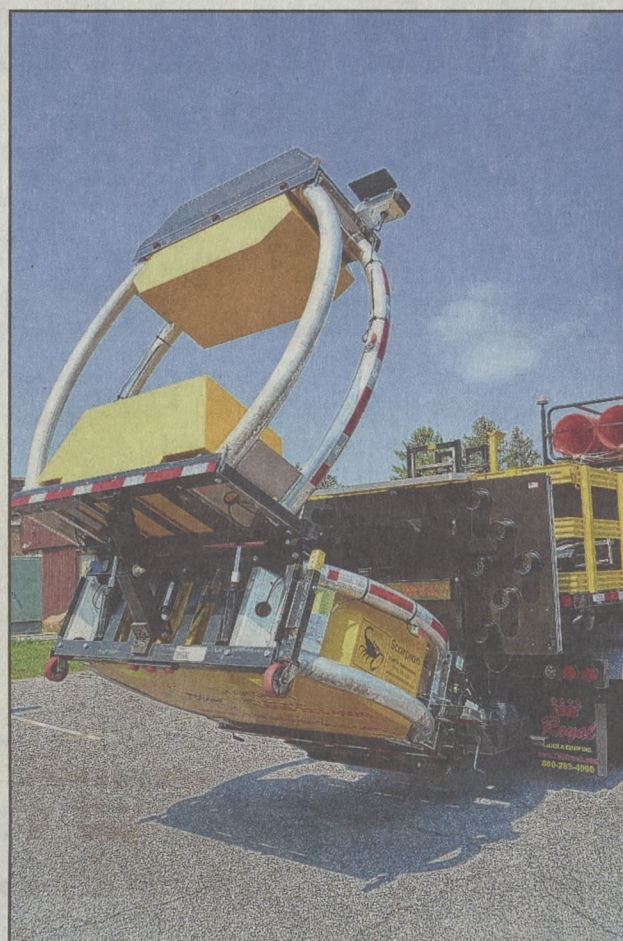
The rear mounted safety alert signal and crash absorption attenuator device folds up and over the ATMA truck body when not in use.
