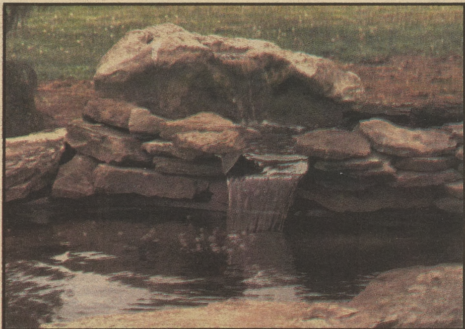
Water falls are made of a concrete and fiberglass composite. Along with adding to landscape design, they stir up water and add oxygen, allowing fish and plants to thrive.
