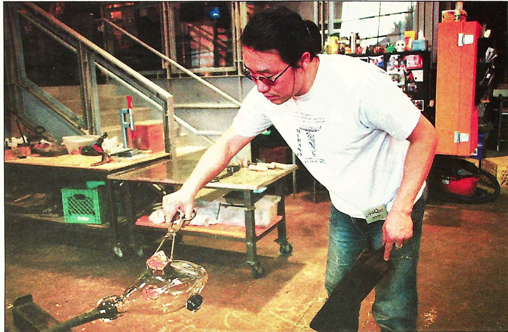
Glass artist John Choi places a piece of hot colored glass on the outside of a sculpture. As it cools, the colored glass will adhere to the other piece.
